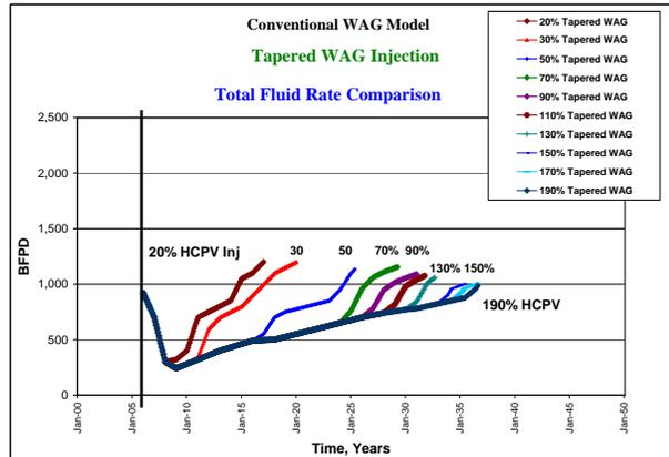
Figure 12b – Total Fluid Rate (Tapered WAG)
