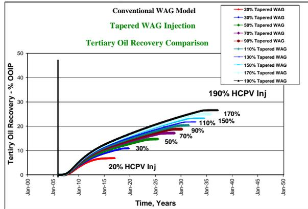
Figure 11b. – Tertiary Oil Recovery (Tapered WAG)
