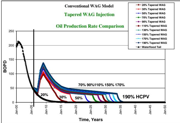
Figure 11a – Tertiary Oil Rate (Tapered WAG)
