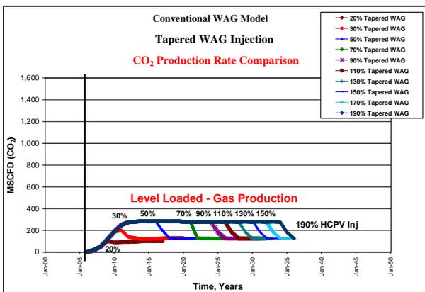
Figure 12a – Tertiary CO<sub>2</sub> Rate (Tapered WAG)
