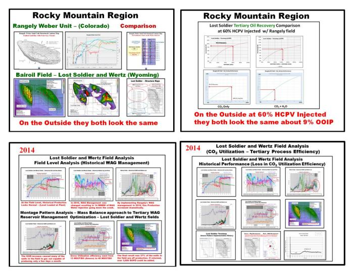
In 2010, Merit Company, who operated the field, modified Amoco's five-spot pattern 9:1 WAG scheme to Rangely's 1:1, 2:1, and 3:1 WAG scheme by dividing the unit up into thirds. From 2010 to 2014, 14 million barrels of water went down the creek that was supposed to be used for WAG Management. The overall effect gassed out 37% of the wells in the Lost Soldier field that deteriated Amoco's Gross  $CO_2$  Utilization WAG efficiency rating of 13 MSCF/BO to over 40 MSCF/BO under Merit's operatorship.
