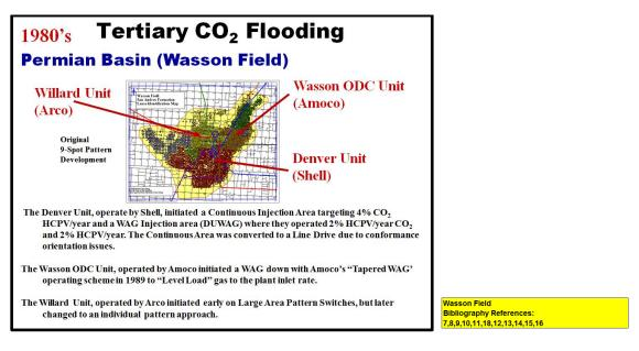
Amoco, in 1989, at the same they implemented Tapered WAG in Slaughter field, implemented a Tapered WAG at Wasson ODC Unit to "Level Load" gas production to its Ryan Holmes Plant Gas Rate Limit. As a result, the benefit of modifying to a Tapered WAG extended Tertiary Oil Recovery way beyond all of Amoco's original model predictions.
