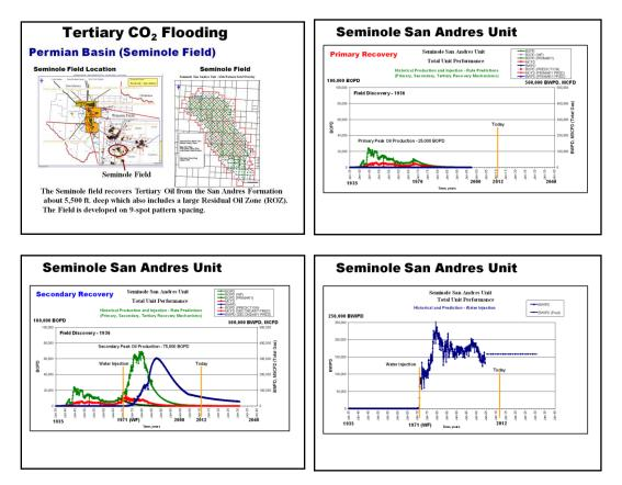
**Tertiary CO<sub>2</sub> Injection operations** into the <u>Main Pay</u> Zone was initiated in 1983. Under CO<sub>2</sub> Injection the field's Main Pay Section is expected to recover an additional 24% of its Original Oil-in-Place (OOIP).
