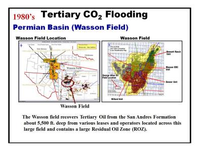
Arco, in the Willard Unit first implemented an area wide switching program based on making large area switches. The reservoir responed with some injectors taking 4% HCPV where others may have had 1% HCPV injected. Due to pattern imbalance issues, Arco then switched to an individual pattern WAG management program.
