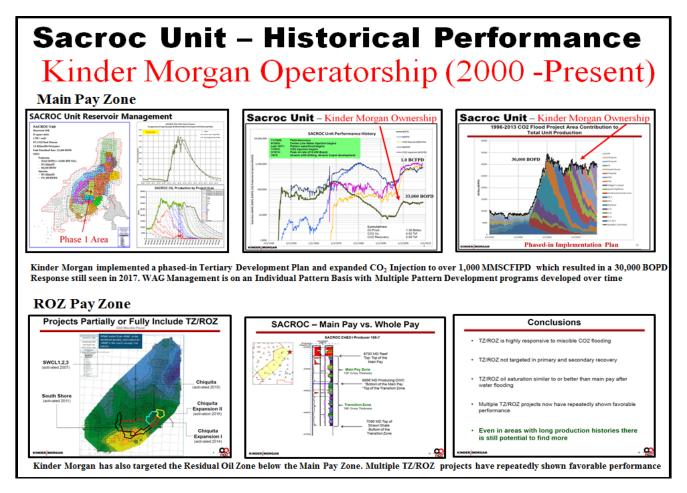
In 2000, Kinder Morgan implemented a multi-phase Tertiary Development Plan that increased  $CO_2$  Injection to over 800 MMSCFIPD, which resulted in a 30,000 BOPD Response still seen in 2017.
